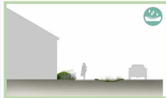
Indicative section through dry swale
