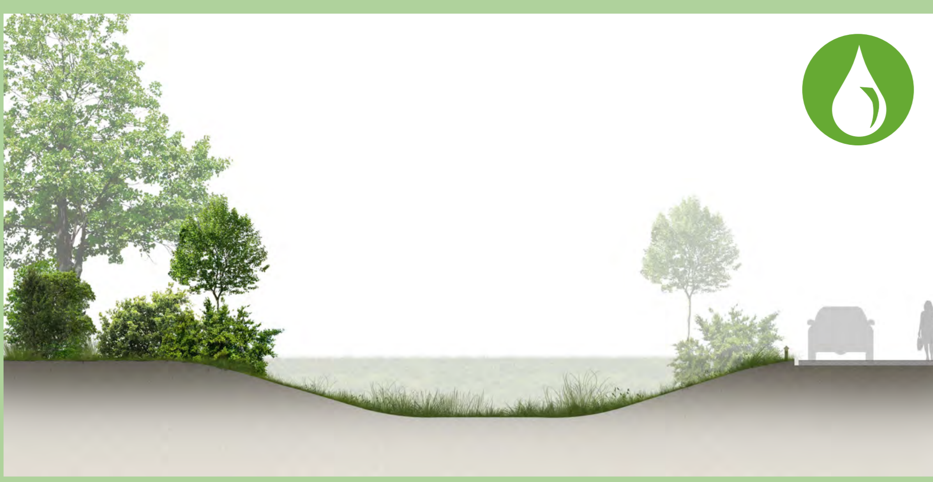
Indicative section through attenuation basin
